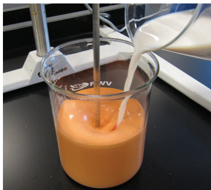
Figure 1. Addition of Kollicoat Smartseal 30 D to Preformulated Additive Dispersion (Step B)
